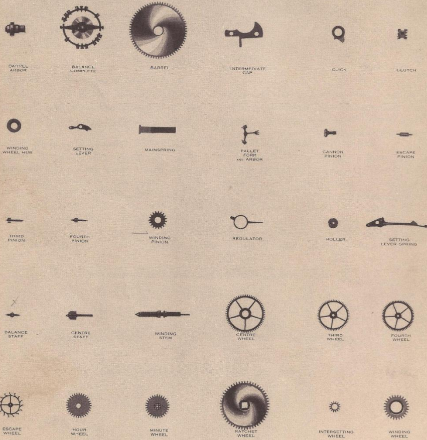
Actual size view of the 18/0 size, Grade 989 movement
